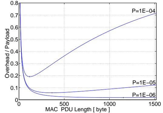
Fig. 4. Optimum MAC PDU length with rest bit errors
