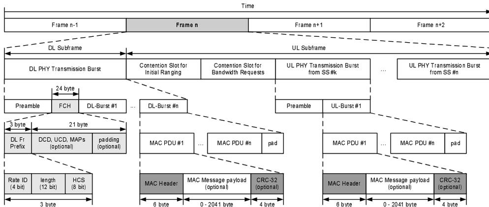
Fig. 2. Frame structure TDD
