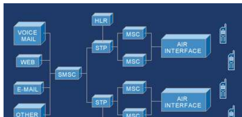
Picture 1. Basic Network Architecture for an SMS Deployment (IS-41)
