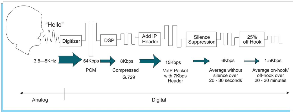
Figure 18 - VoIP Bandwidth Reduction Sequence
