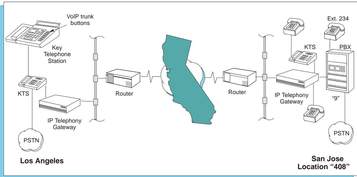
Figure 12 - Calling from a KTS using VoIP
