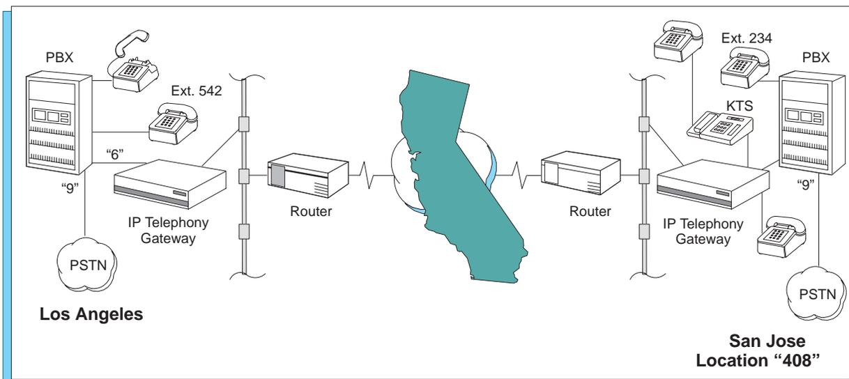
**Figure 11 - Calling from a PBX using VoIP**
