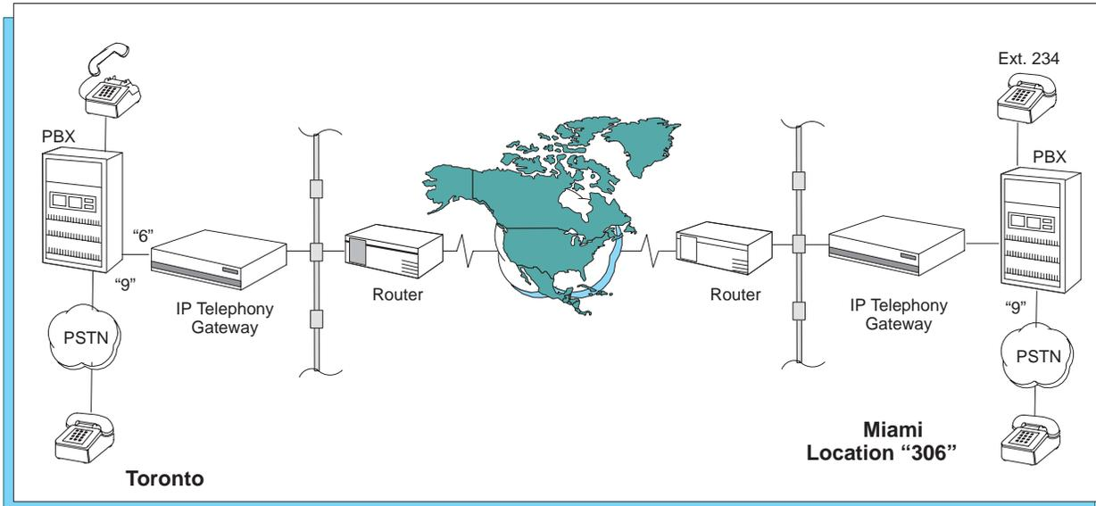
Figure 14 - Off-net calling using VoIP
