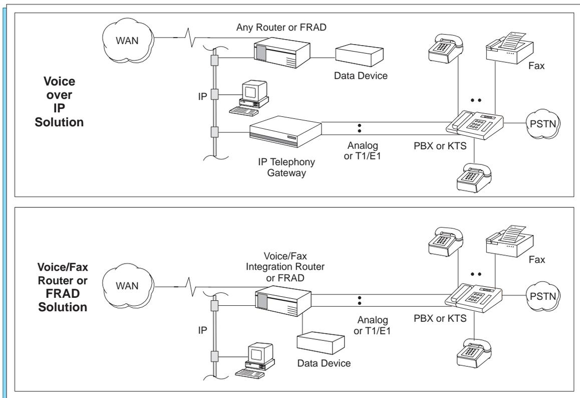
Figure 10 - Comparing VoIP Gateway with Voice/Fax Router or FRAD
