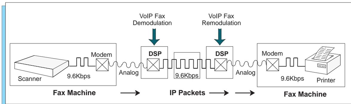
Figure 8 - VoIP Fax Demodulation/Remodulation at 9.6 Kbps
