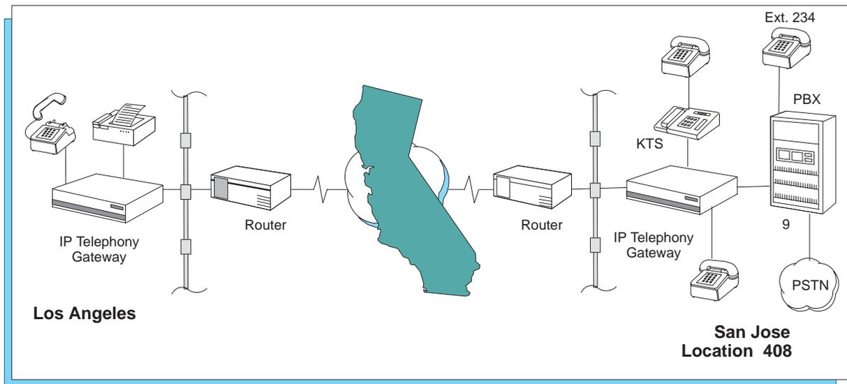
Figure 13 - Calling from a directly connected phone using VoIP
