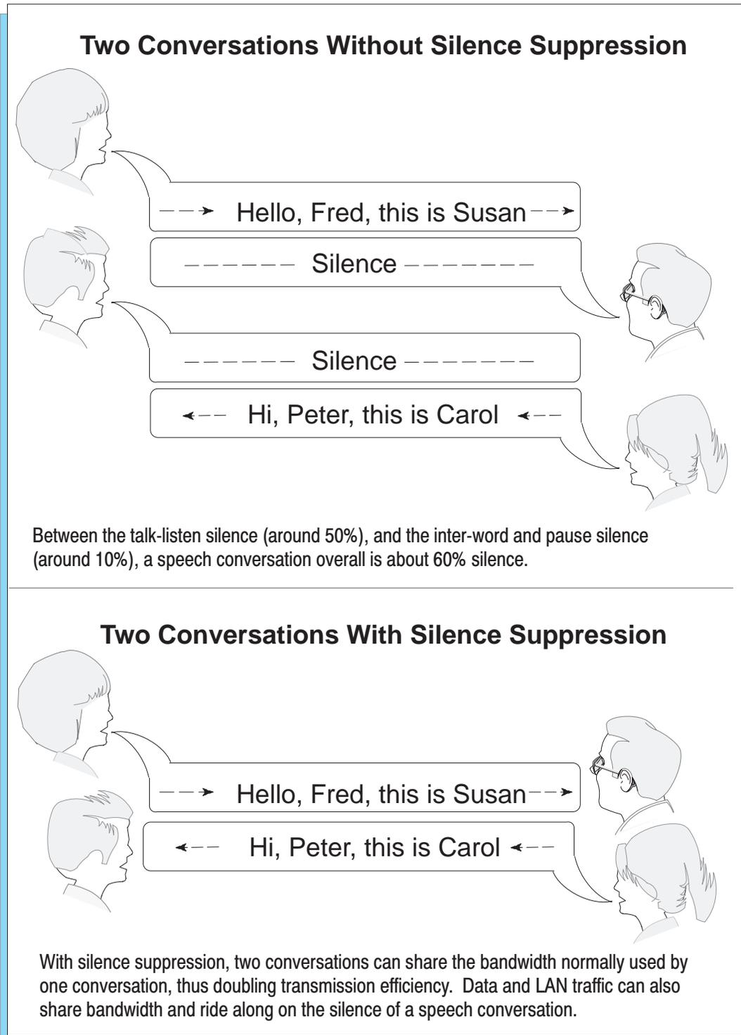
Figure 17 - Conversations with and without Silence Suppression
